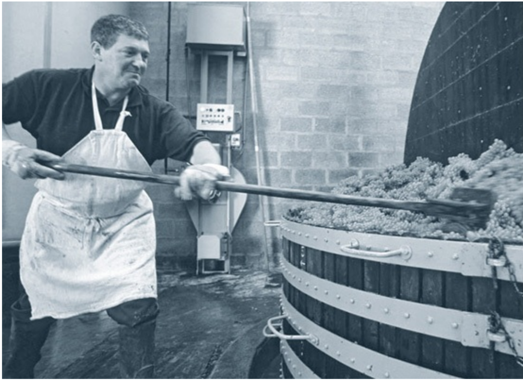
In Champagne, a traditional basket press is often still used for grapes.
