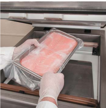
4 Placing the whole salmon terrine into the chamber vacuum machine, which will help it hold its shape.
