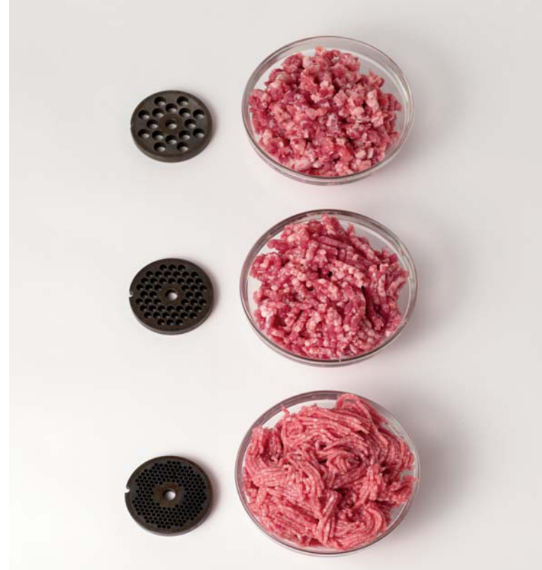
Progressively ground meats, from top to bottom: coarse die, medium-coarse die, small die.
